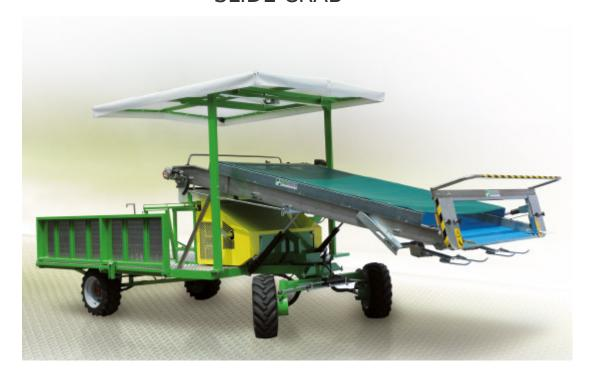
SLIDE CRAB is the perfect harvesting machine for the harvest of baby-leaf, rucola, spinach and all leaf vegetables grown in greenhouses or in open field. SLIDE CRAB is featured, if compared with the standard version, both by a strong structure and a loading capacity of approx.1000-1200 kg. The most innovative features are its hydraulic system of the latest generation and the four steering wheels, that make easier the maneuver, also in small spaces.
